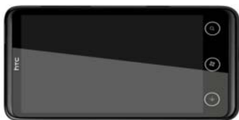
Fig. 2 Shows the solution to the problem. All buttons have a proper boundary defined and shows a circular region around every button
